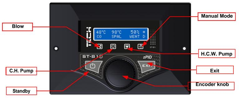
The **ST-81i** temperature regulator is intended for use with central heating boilers. The regulator is used for controlling the central heating water circulation pump, hot consumption water pump and blow (fan).
